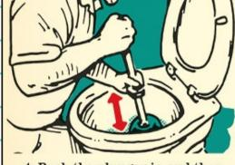
4. Push the plunger in and then release, allowing it to pop back out. Make sure the tight seal is maintained during both directions of movement.
