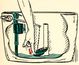
1. Stop the bowl from filling further by removing the top of the tank and pressing the flapper down.
