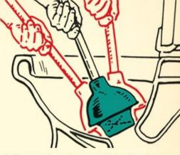
Press the plunger into the bottom of the bowl, taking care to ensure a tight seal is formed.
